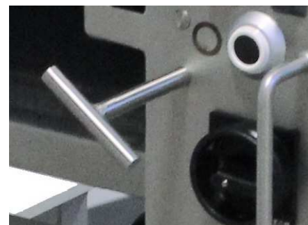
ThinAdjust Control allows for the skinning thickness to be adjusted during operation, resulting in consistent yields and final product.
