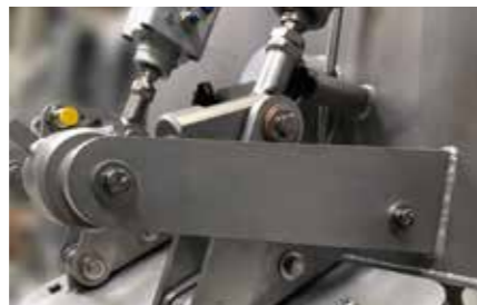
Pneumatically operated discharge gates with strong knee-lock.
