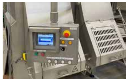
Pivoting digital operator panel mounted on a swivel arm.
