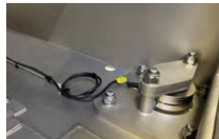
The weighing cells are mounted inside the main cabinet, protected from cleaning and water spray.
